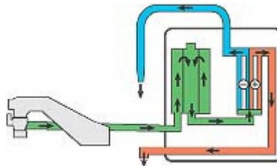
A special attachment redirects tap water out of the faucet through a plastic hose into the Microwater unit. Inside the Microwater unit, the water is first filtered through activated charcoal. Next, the filtered water passes into an electrolysis chamber equipped with a platinum-coated titanium electrode where electrolysis takes place.
